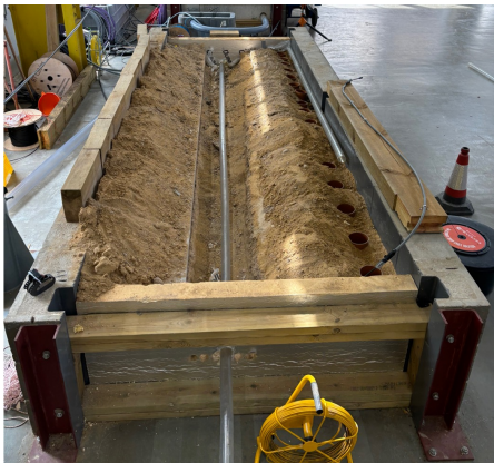
Figure 4.11: BT OpenReach fibre optic cable duct testbed, featuring two 3m x 50mm ID cable ducts connected by a spigot and socket joint.
