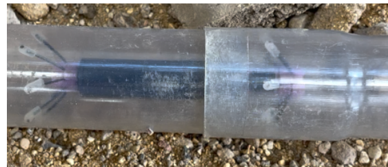
Figure 4.12: Inchworm prototype stuck in the spigot and socket pipe joint
